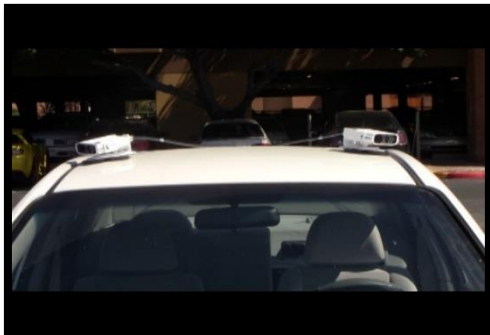
LPR camera equipment
